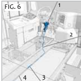
Fig. 6 1. Parking brake assembly 2. Front Cable 3. Adjustment turnbuckle 4. Intermediate cable
