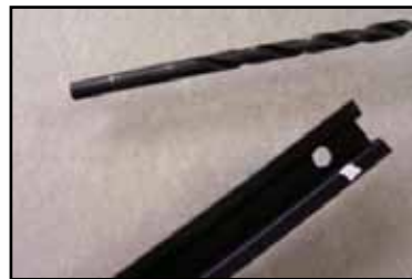
Drill a 3/16" hole in the plastic guide.
