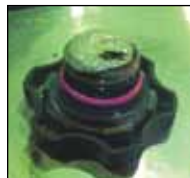
Figure 3: Sludge on breather cap
