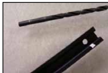
Drill a 3/16" hole in the plastic guide.
